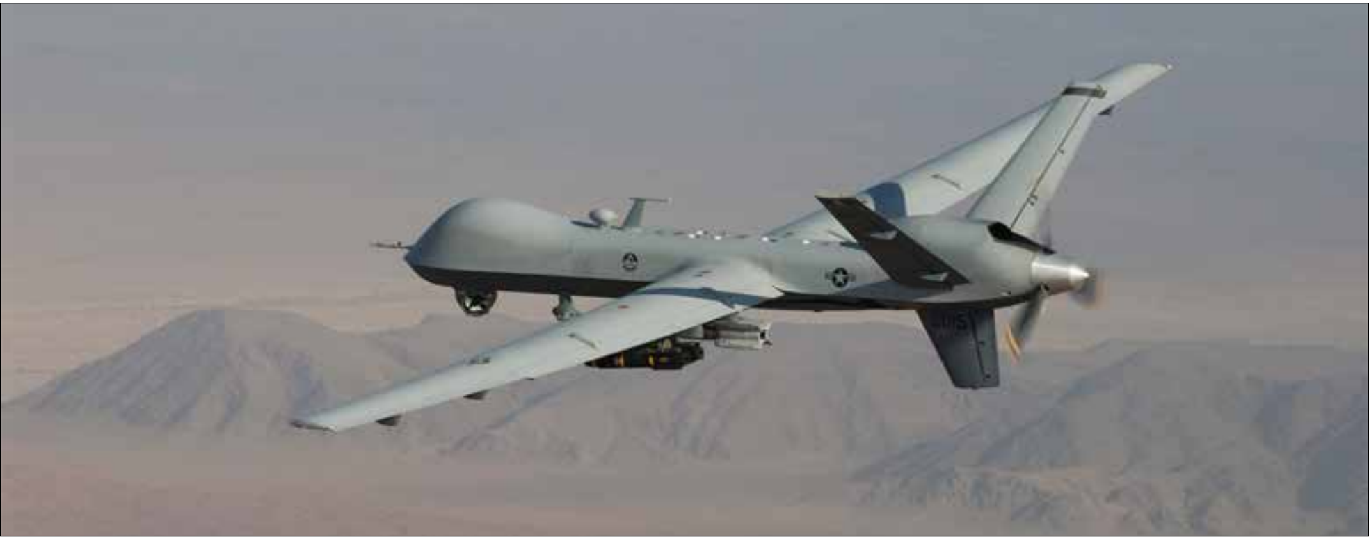
An MQ-9 Reaper, armed with GBU-12 Paveway II laser guided munitions and AGM-114 Hellfire missiles, piloted by Col. Lex Turner flies a combat mission over southern Afghanistan. (U.S. Air Force Photo / Lt. Col. Leslie Pratt)
